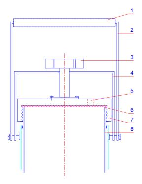
Component parts of lid without overpressure valve (Special designed)
