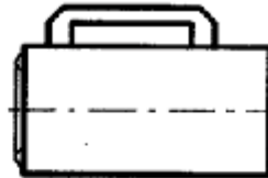
Type "G-C" standard cover ALU smooth blue coated with handle
