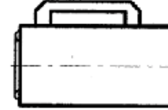
Type "G-C-E" special design, cover made of stainless steel with handle
