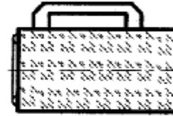
Type "G - CAL" special design, cover ALU Stucco with handle
